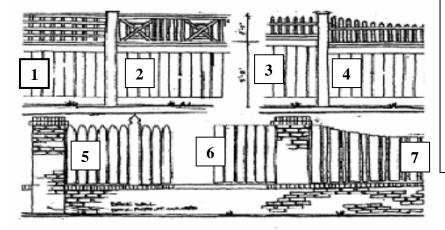
Styles 1-4 are 1x4 board on board with 2' non-solid caps and 6x6 Posts. Slats may be 1x6 if desired.
